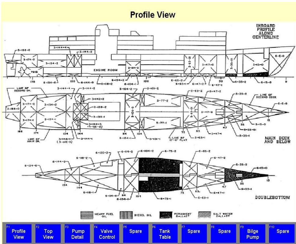
Figure 3. Ballast System Control Screen (Tank Arrangement)
