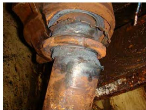
Figure 1 Destroyed shaft line at high speed due to whirling vibration
