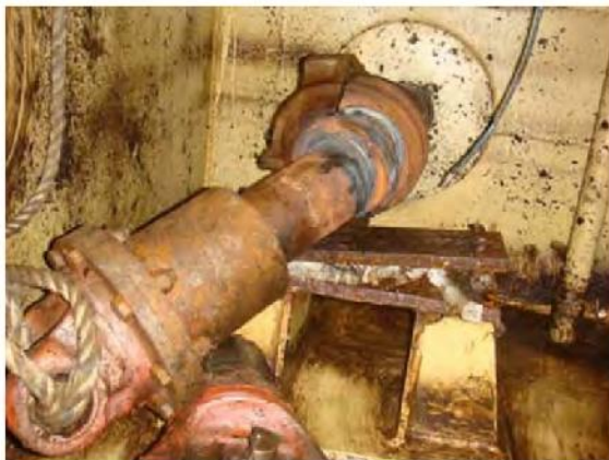
Figure 1 Destroyed shaft line at high speed due to whirling vibration
