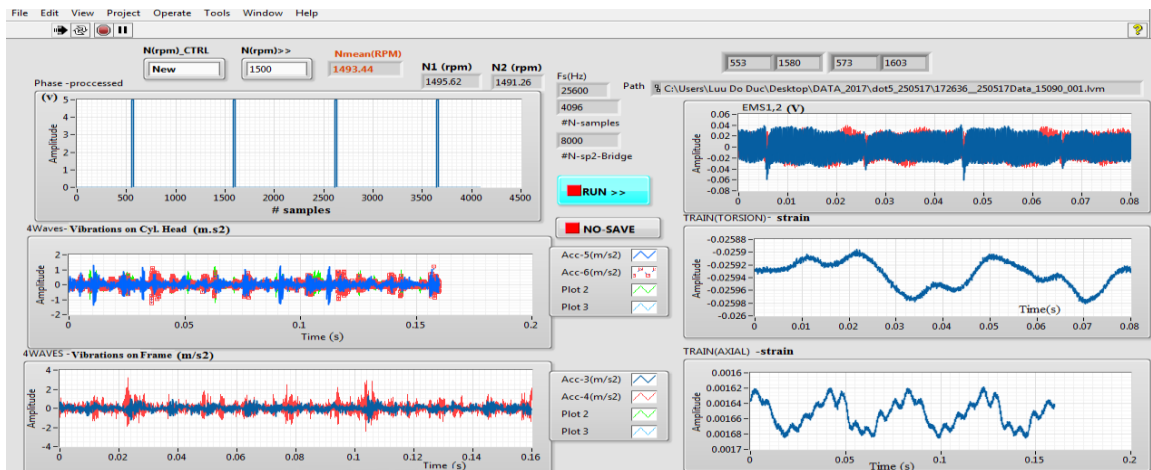
Fig.4 Express data processing and monitoring measurement vibrations on D-G set 110 kW using MVMS, experiment regime N=1500 rpm, I=100A (Load)
