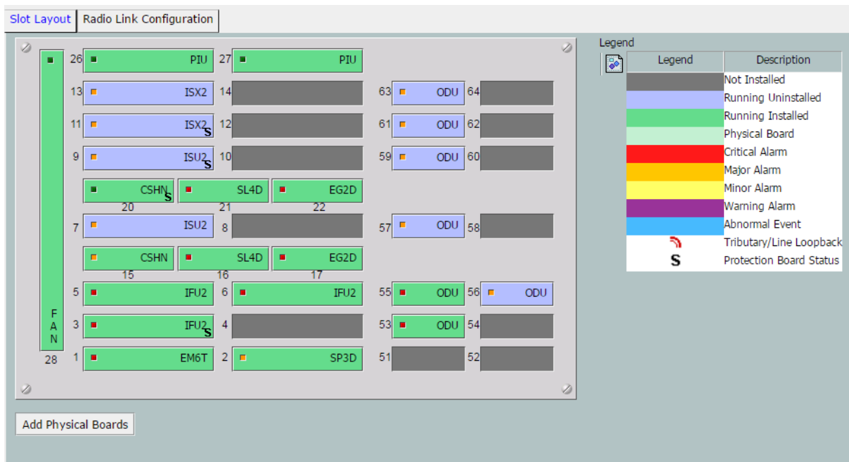
Fig.4 Slot layout of the microwave equipment Optix RTN980
