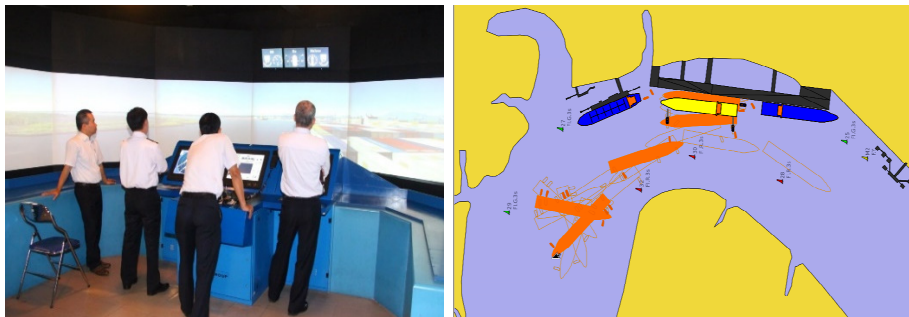
Figure 3: Manoeuvring test of 14,000 TEU container ship at Tancang-Caimep
