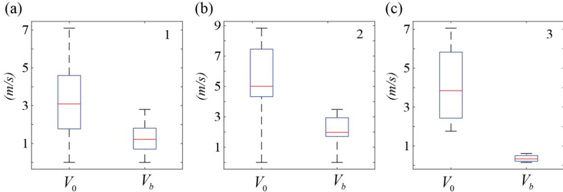
**Figure 4.** Efflux velocity and bed velocity results for the maximum potentially harmful instants according to Figure 2. (a) Arrival -1. (b) Departure -2. (c) Departure -3.
