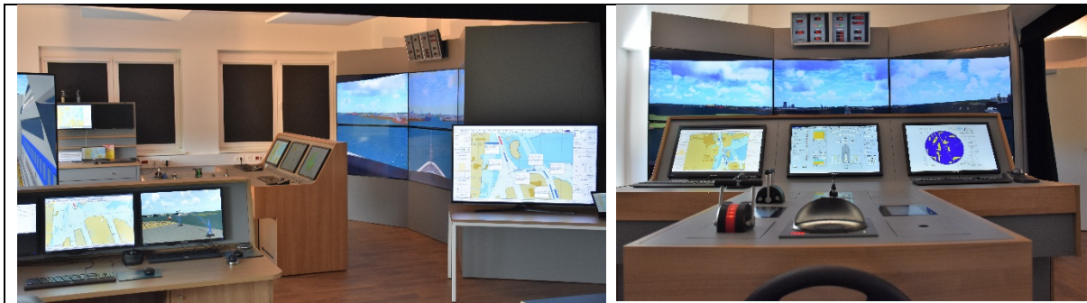
Fig. 2 ANS 6000 brige simulator with Fast Time Simulation System for Simulation-Augmented Manoeuvring Design, Monitoring & Conning - SAMMON is fully integrated to the ANS 6000 by a smart interface using LAN and WLAN
