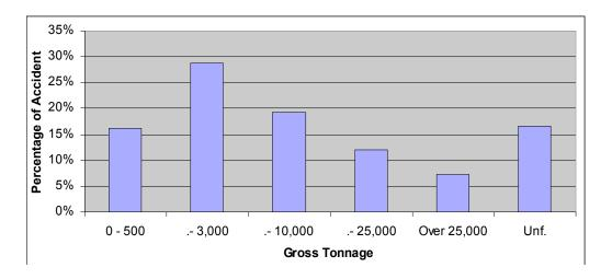
Fig. 12 The percentage of accidents based on the ships' tonnage
