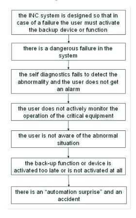
Fig. 2 The chain of events of a typical accident due to a fault of the INC system
