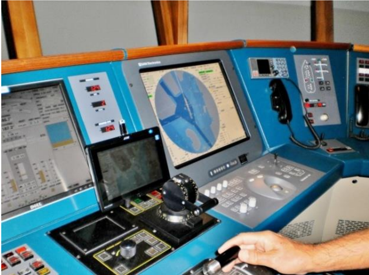
Fig. 6: Portable setup for prediction display on ECDIS in Monitoring Tool on students laptop on bridge 1 of ship-handling simulator of MSCW – the prediction is controlled by the bridge handles. The dynamic prediction shows the future manoeuvring track whereas on the radar screen the static path prediction shows still a straight line according to the initial conditions of the ship-handling simulator of MSCW.
