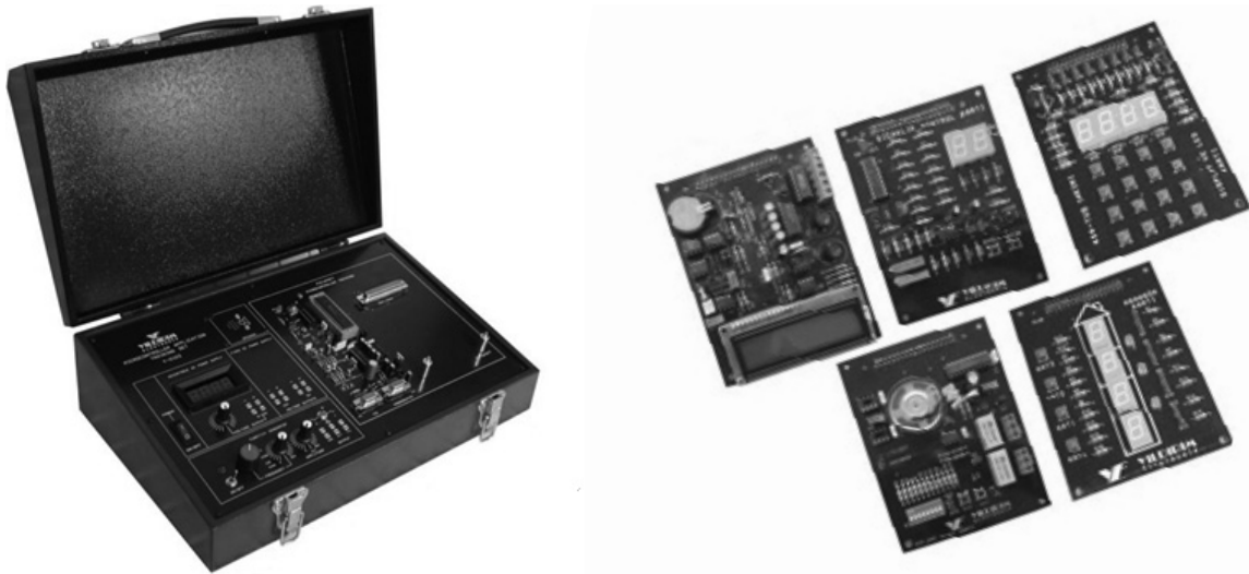
Figure 3 Microprocessor Training Set and Application Modules
