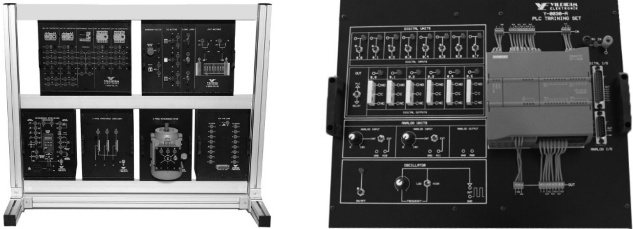
Figure 1 PLC Training Set at ITUMF Mechatronics Laboratory
