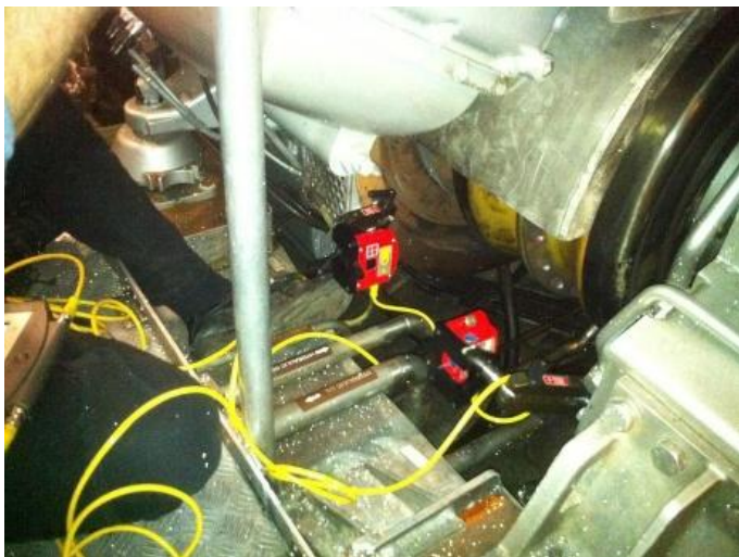
Figure 3 – Dynamic movement set up on Vessel x
