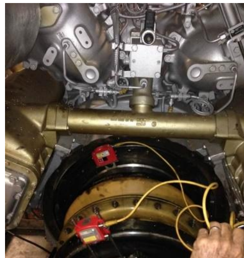
Figure 4 – Shaft alignment on Vessel x
