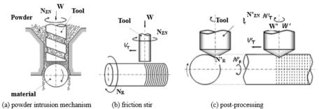
Figure 1. Method of friction reforming
