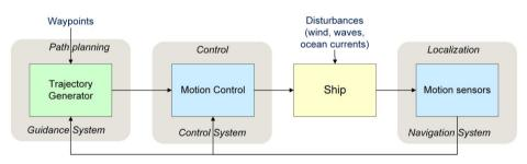
Figure 1. Guidance, Navigation and Control system.
