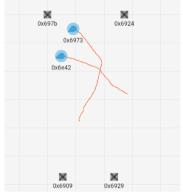
Figure 3. Results of experimental studies for an encounter situation with one dynamic obstacle registered with the use of an Indoor Positioning System.
