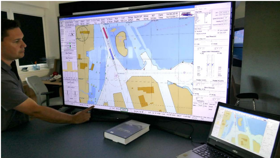
Fig. 7: Fast time planning in sea chart on a big touch screen or on a laptop: Initial ship position (red shape) at MP0 is set with adjusted heading and rudder angles to balance the wind 10kn from 61°. The prediction (black dotted shapes) shows the motion of the ship due to the handle setting on the right window. The ship is moved as blue shape by the time slider at the bottom from MP0 to the next position to be set as following MP1
