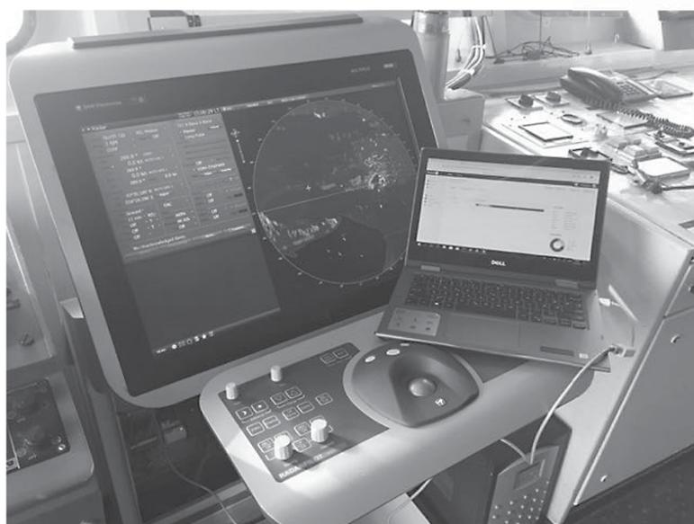
Figure 2. Computational cyber vulnerability scanning of the ship's chart-radar system.
