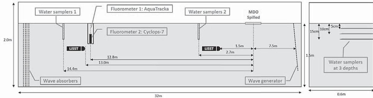
Figure 1. Schematic drawing of the wave tank (not to scale, all values are in meters) for surface oil release tests.
