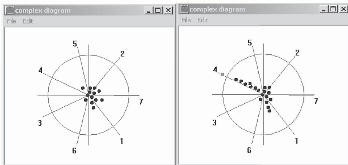
Fig. 2: Complex diagram without/with disturbance on cylinder 4
