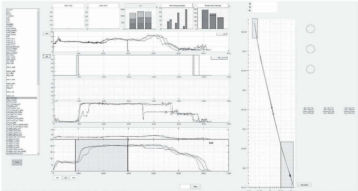
Figure 1 Ship's data analysis software allows for prediction of fuel consumption and emissions for a single manoeuvre, manoeuvre sequences or for a whole voyage "pier to pier" on the basis of available navigational and engine data. The post-processing algorithm enables to analyse the energy management and its efficiency.
