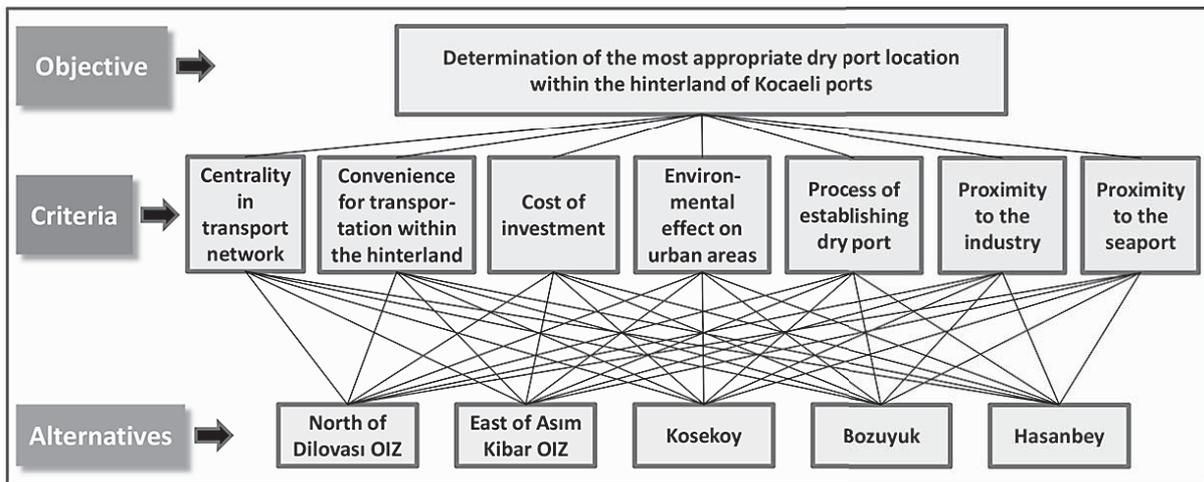
Figure 2. AHP plan to determine the most appropriate dry port location.
