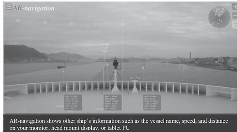
Figure 1. Prototype of mixed (augmented) reality interface
