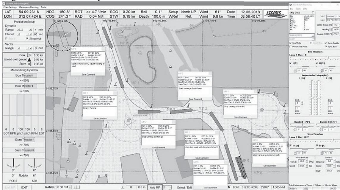
Figure 2 Sample for complete manoeuvring plan with final stopping manoeuvre and berthing by thrusters; additional manoeuvring point information text boxes show the control setting for the briefing session
