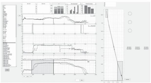
Figure 1 Ship's data analysis software allows for prediction of fuel consumption and emissions for a single manoeuvre, manoeuvre sequences or for a whole voyage "pier to pier" on the basis of available navigational and engine data. The post-processing algorithm enables to analyse the energy management and its efficiency.
