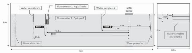
Figure 1. Schematic drawing of the wave tank (not to scale, all values are in meters) for surface oil release tests.
