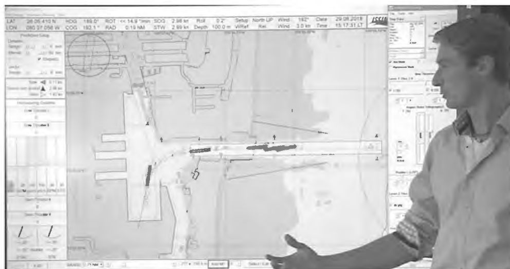
Fig. 4 Manoeuvring Design & Planning Tool Demonstration: Planning of manoeuvring sequence for a cruise vessel for arrival at Ft. Lauderdale by Nautical Officer of AIDA Cruises on touch screen.
