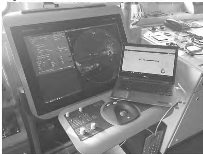
Figure 2. Cyber security testing of the chart-radar.
