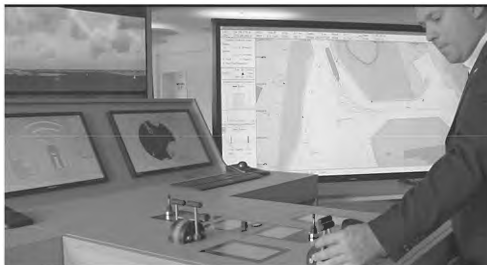
Fig. 5 Manoeuvring Monitoring & Conning Module – Demo of using bridge handles in to train “Touch and Feel” for Controls with Multiple Dynamic Prediction showing the effect of any control change immediately as future ship shape on ENC (SAMMON Demo on Bridge Simulator at benntec / Marinsoft Office at Rostock-Warnemünde Germany)
