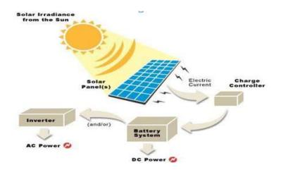
Figure 4 photovoltaic solar power arrangements
