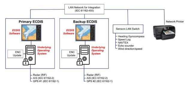
Figure 1: Primary and backup ECDIS arrangement
