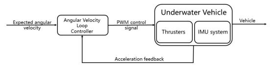
Figure 5. Structure of single-stage angular velocity PID controller
