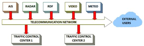
Figure 1. Typical VTMIS Architecture
