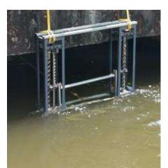
Fig. 3. Field test of HVPG Module Phase III at Palissery irrigation canal
