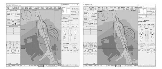
Figure 6: SAMMON planning interface: Starting position at MPO and predicted shapes for the following slow down manoeuvre beginning at MP1: Left:: in conventional way with reducing EOT to 10%; right: turning both pods inward IN 30°
