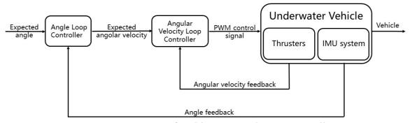
Figure 4. Structure of multi-stage angular PID controller
