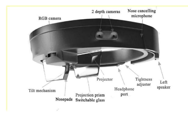
Source: https://mspoweruser.com/instead-of-5-cameras-hololens-2-0-may-just-have-one/ Figure 2: HoloLens (OHMD)
