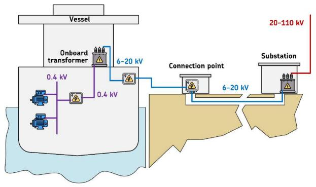
Figure. 1. General arrangement of cold ironing [2][1].
