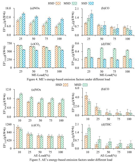
Figure 4 and 5 show that the energy-based emission factors are closely related to the diesel engine type and load. The diesel engine operated under low load will lead to a higher NOx energy-based emission factor. This is because when the diesel engine works at low load, the amount of fuel injection per cycle is reduced, but the oxygen content in the cylinder is increased,
