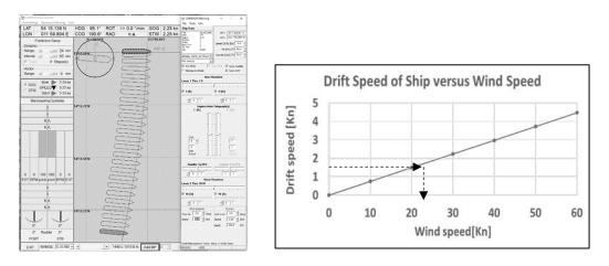
Figure 2: Transverse Drifting under Wind speed VA=30kn (Cruise ship AIDAblu). Left: situation with drift speed SOG=2.25kn, HDG 94°, COG 184°; right: diagram for drift speed versus wind speed with arrows indicating maximum drift balance by thrusters
