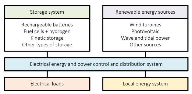
Figure 2 Schematic diagram of marine port power supply system microgrid concept [6], [1].
