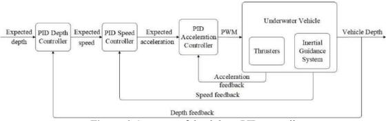
Figure 6. Structure of depth loop PID controller
