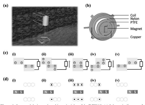
**Figure 1.** Structural design and working principles of the T-TENG. (a) Schematic diagram of the designed H-WEH consisting of multiple units. (b) Exploded view of the H-WEH's structure. (c) The working principle of the TENG component. (d) The working principle of the EMG component.
