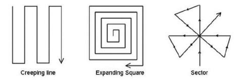
Figure 1: The standard search patterns as per the IAMSAR Manual: creeping line, expanding square and sector search [1].
