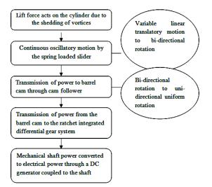
Fig.2. Flow diagram of power transmission system
