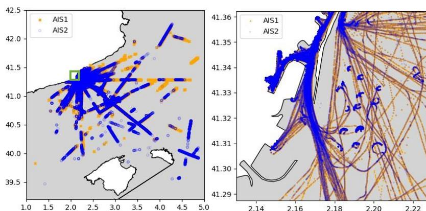
Figure 2. Geo-positional AIS received messages in June 1<sup>st</sup>, 2021. AIS1: old antenna, AIS2: new antenna. Left: all data received; right: zoom in the green square in left figure
