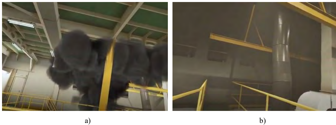
Figure 8. Smoke on the upper deck of the engine room: a) VR generic, b) CFD-based.
