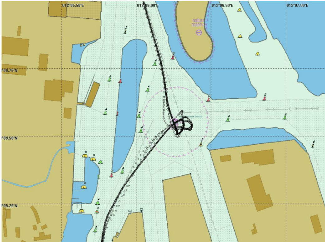
Fig. 103: Recorded tracks of real harbour manoeuvres of a ferry
