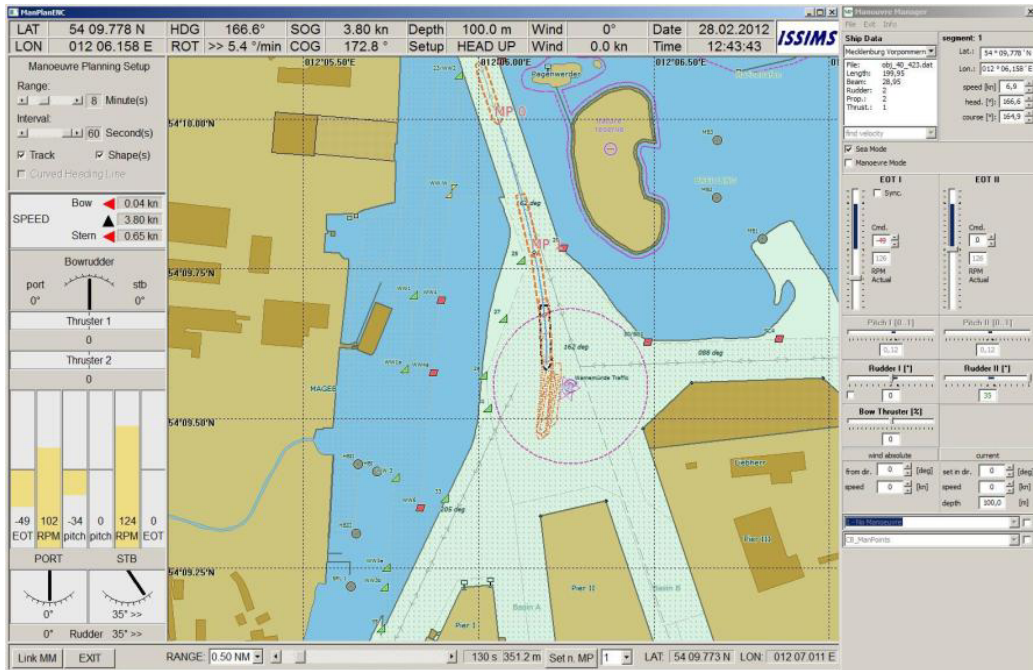
Fig. 94. Planning of the next segment from MP 1 to MP 2 – speed reduction
