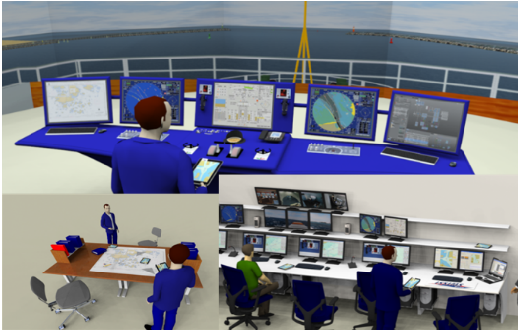
Fig. 97. SAMMON System set up based on Tablet PCs within Ship Handling Simulator environment: as Bridge Version (top), Lecturer System (left) and Instructor Version (right)
