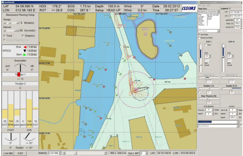
Fig. 95. Planning of the next segment from MP 2 to MP 3 – complex turning and stopping with engines, rudders and thruster
