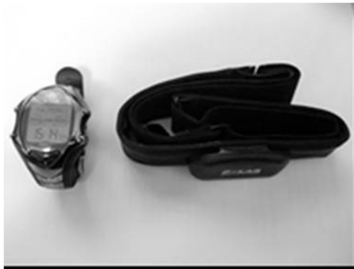
Fig. 5. The heart rate monitor, wrist watch and chest belt
