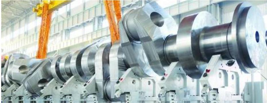
Fig. 1. Typical ship engine crankshaft
