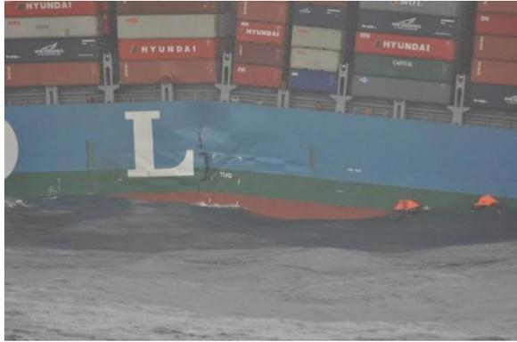
Fig.3 Damage extent (detail)
