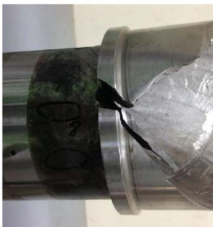
Fig. 2. Shaft crack detail
