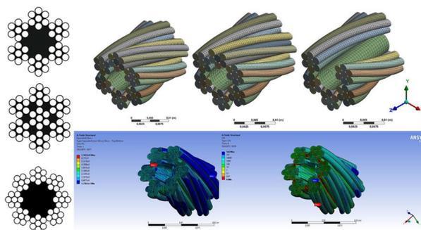
Fig. 5.1 Numerical analysis of remaining fatigue life of a wire rope
