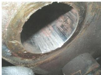
Fig.3 Coupling between intermediate and tail shafts (detail)
