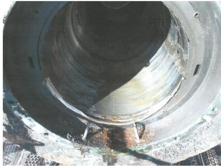
Fig. 1. Condition of aft and fore of stern tube bearing
