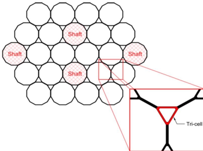
Fig. 2. Plan view of SLA-1 buoyancy cells
