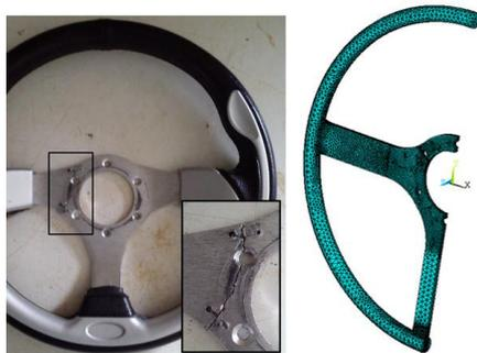
Fig. 7.3.1. Numerical model of fractured speed boat steering wheel.
