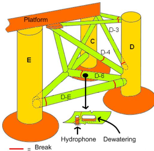
Fig. 2. Fractures on the rig
