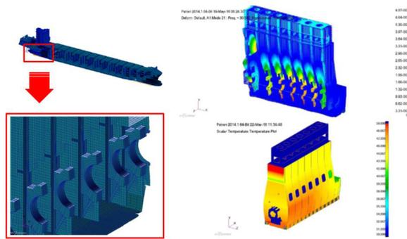
Fig. 3.1. Numerical model of the engine body-ship hull interaction and thermal loads presenting a threat to structural integrity [7]
