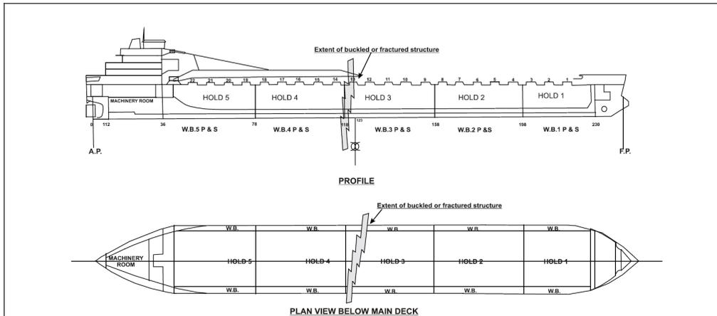
Fig.3 Damage location
