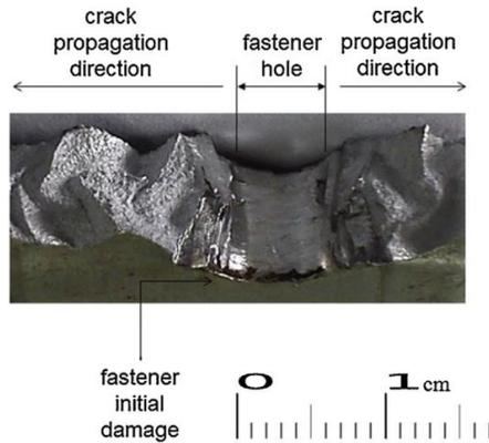
Fig. 2. Crack detail
