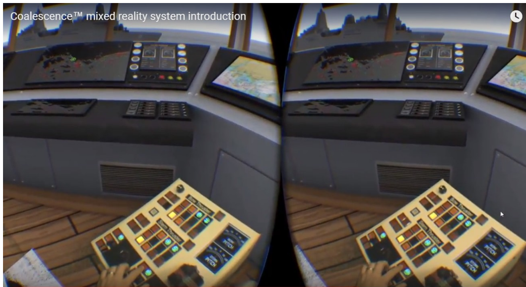
Figure 4: Mixed reality. View through a VR headset. The real consoles with hands are combined with a virtual ship bridge with ECDIS, radar, windows and outside view.
