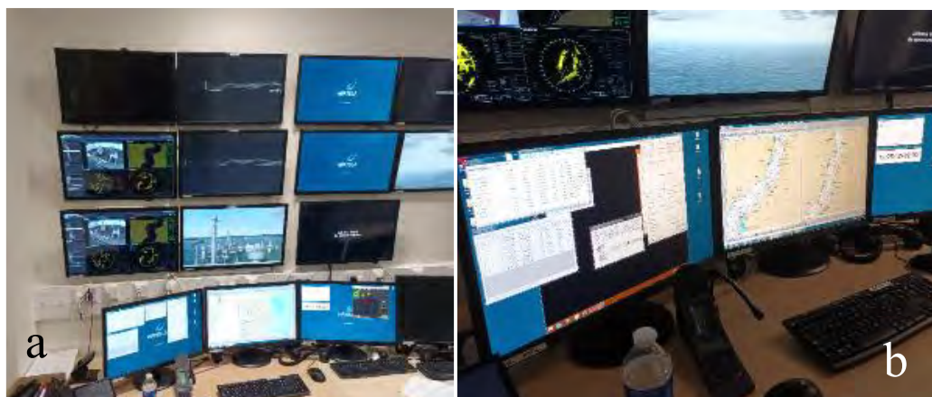
Figure 30. a) Wall monitors in the instructor suite to observe and hear activity in each simulator through CCTV, as well as ECDIS and RADAR screens, and b) Desk monitors to view specific screens such as ECDIS and Radar, as well as the monitor the proximity of traffic, ship dynamics, ship logs, and ship forces.
