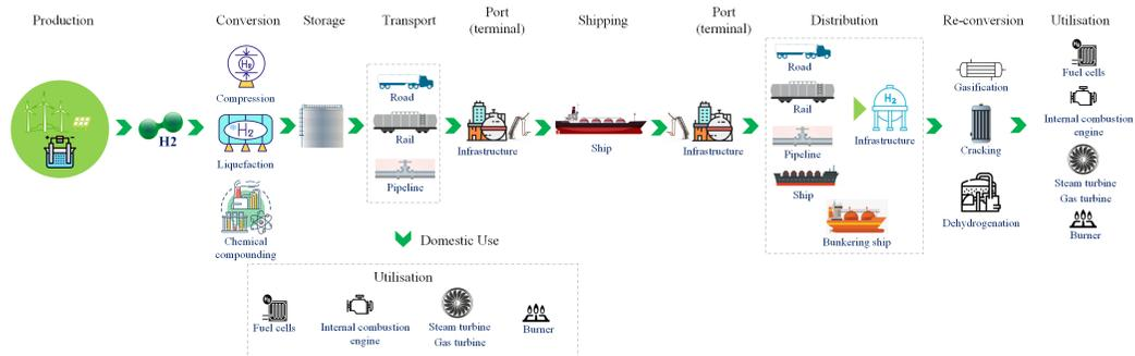
**Fig. 6 Hydrogen supply chains**
