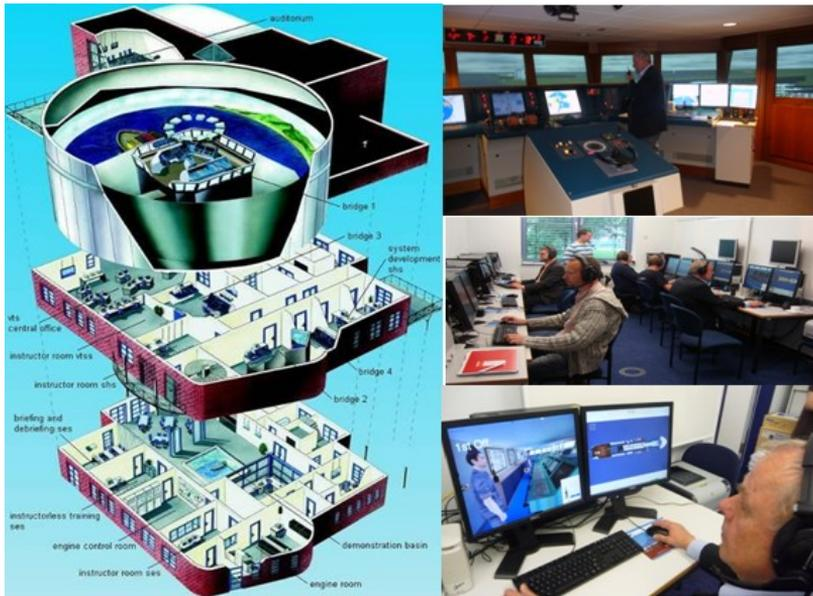
**Figure 11.** Overview on MSCW (left), Bridge 1 of Ship-Handling-Simulator (SHS) with new Displays of Bridge Safety & Security Centre of SST and MADRAS Decision Support System (right top) and Training room of new Safety & Security Trainer of SST (right bottom)
