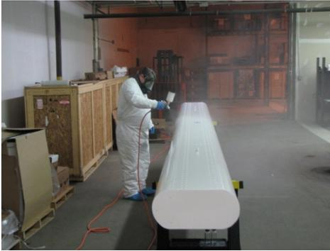
**Figure 7.** Application of PCM
