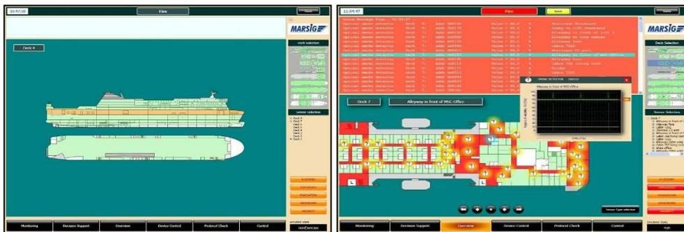
Figure 9. MADRAS – Overview of deck and installed sensors, diagram of activated sensor
