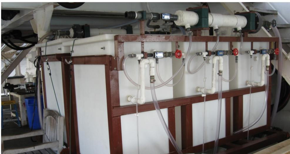
**Figure 4.** Slip Stream Sampling System
