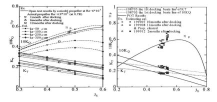
Figure 5: Propeller performance of "Fukaemaru" in service.
