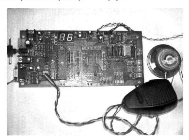
Figure 6: VHF circuit board connection.
