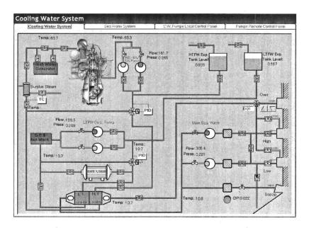
Figure 9: A MMI of cooling water system.
