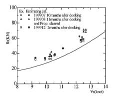
Figure 6: Hull resistance of "Fukaemaru" in service.
