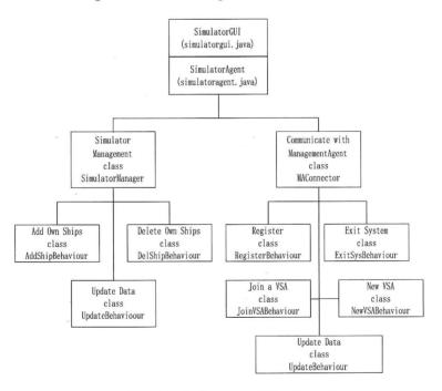
Figure 3: Block diagram of Simulator Agent.
