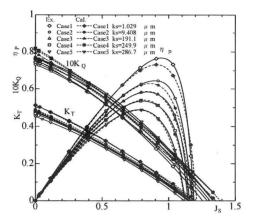
Figure 3: Experiment results of fouled propeller performance.
