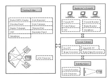
System configuration of the second onboard SMS. Figure 10:
