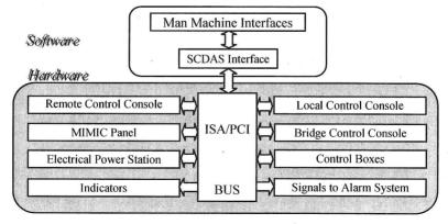
Figure 2: Data acquisition and control system.
