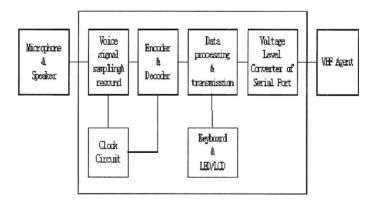
Figure 5: VHF Terminal Architecture.
