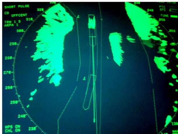
**Fig. 3 The predictor on the radar screen**
