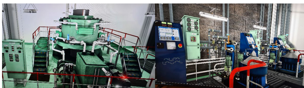
Figure 4. Steering gear and the purifiers in the marine engine room simulator (left to right).
