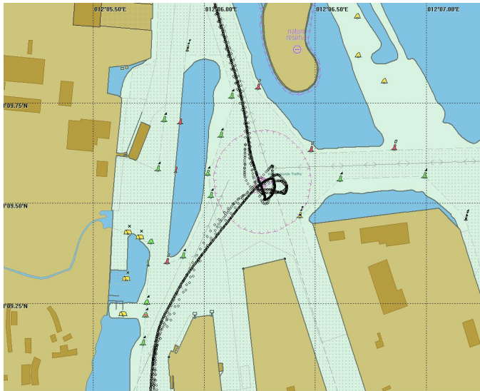
Fig. 12: Real track of harbor maneuvering of MV „Mecklenburg-Vorpommern“, based on VDR (high spot density), and recorded AIS information
