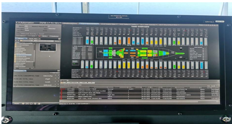
Figure 4 - M/S AURORA BOTNIA tank overview. (Source Heikki Koivisto)
