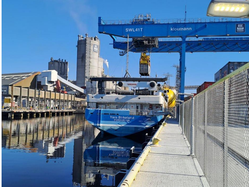
Figure 11 - YARA BIRKELAND loading full containers at their homeport Porsgrunn. (Source Heikki Koivisto)
